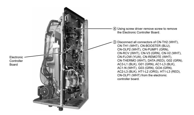
17.7. To Remove Pressure Relief Valve, Flow Switch, Water Pump and Bottle Complete
