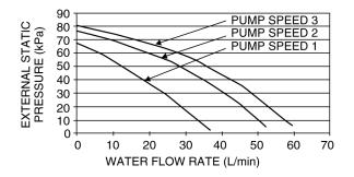
• Flow rate characteristic of indoor unit is as per above mentioned.
