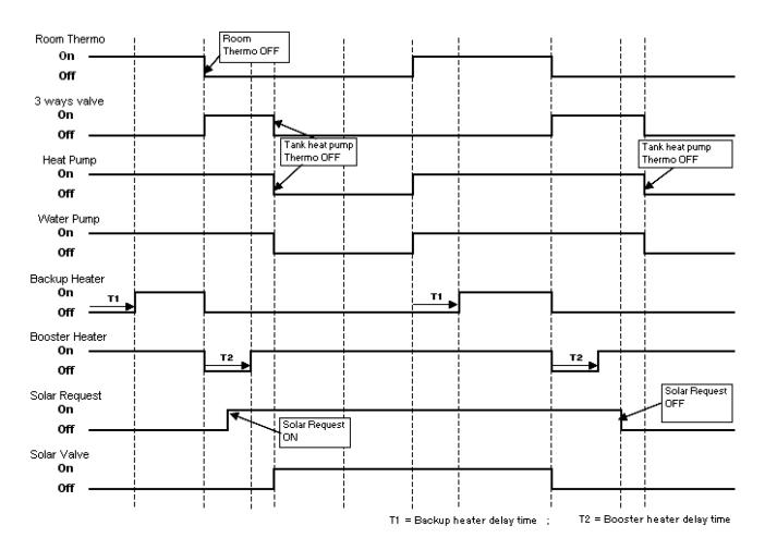
Setting 2:- When heating priority is not set by control panel: • When Solar Priority is set / not set by control panel:
