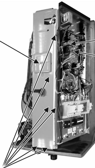
① Disconnect the connector of CN-REMOTE (WHT) from the Electronic Controller Board.
