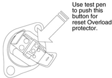
Use test pen to push this button for reset Overload protector.
