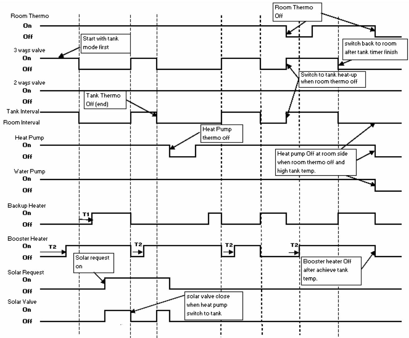
T1 = Backup heater delay time ; T2 = Booster heater delay time
