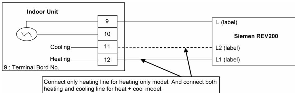
Wire Connection and thermo characteristic of Siemen RAA20:
