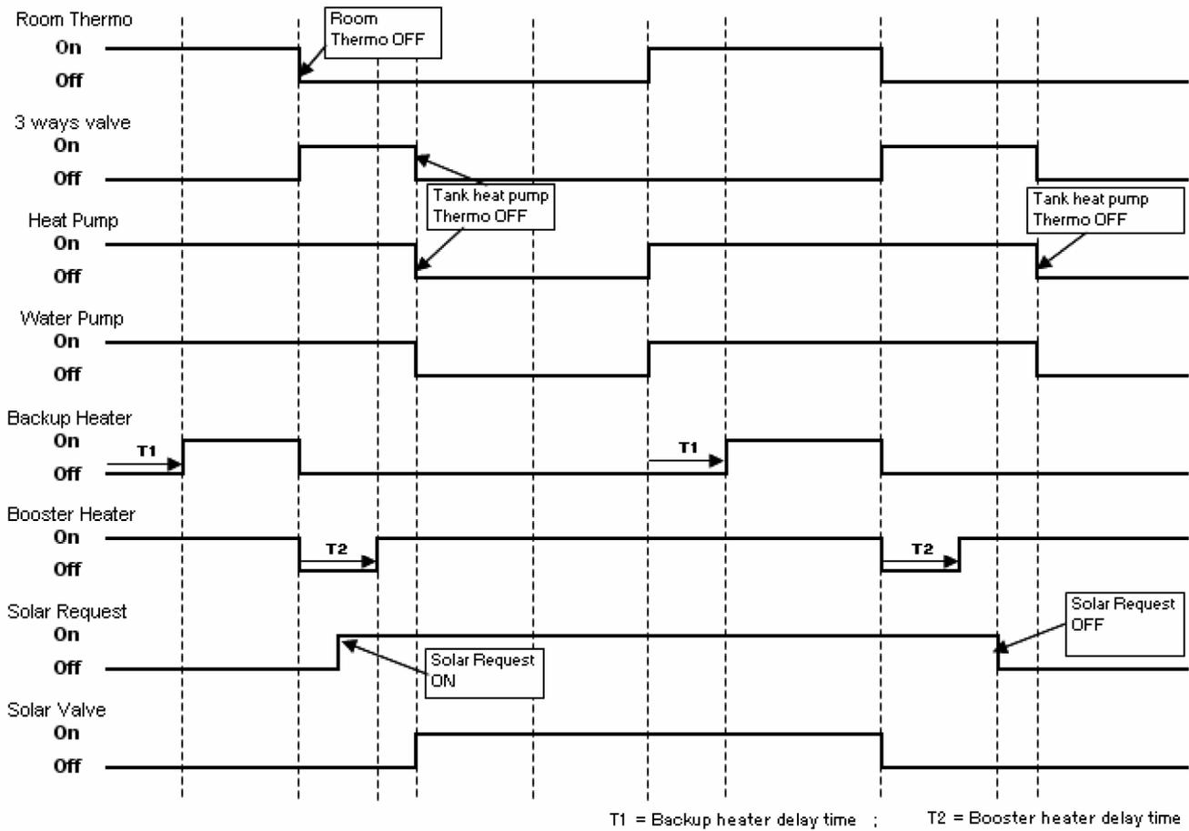
Setting 2: When heating priority is not set by control panel:
